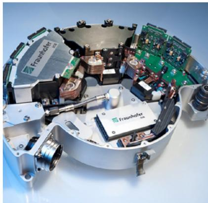
An SiC inverter for a smart, compact, modular, and durable in-wheel drive unit was developed at Fraunhofer IISB. The inverter provides easy servicing of the complete powerstage due to a plug-and-play interface, good manufacturability, and flexibility. This helps to increase the availability of hybrid and electric vehicles, which is essential for commercial use. Main component of the modular integration approach is a newly designed Inverter Building Block (IBB).
