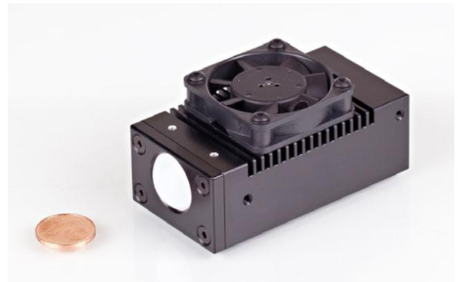
The new high frequency radar scanner can monitor its environment in a 360-degree radius with a precision of less than a micrometer and a transmission range of up to several hundred meters. It also shines through optically intransparent materials such as smoke, fog, paper, boxes, or plastic boards.
