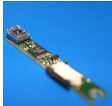
Fraunhofer ISIT has developed a 3D camera based on a 2D MEMS scanner, which uses the principle of phase difference of a laser beam to the detected “echo” as distance measurement. The phase detection algorithm allows 60 million 3D measurements per second. The camera has a resolution of 450 × 450 pixels and provides six images per second. The depth resolution is a few millimeters and the maximum detectable distance to the object is 2 m.
