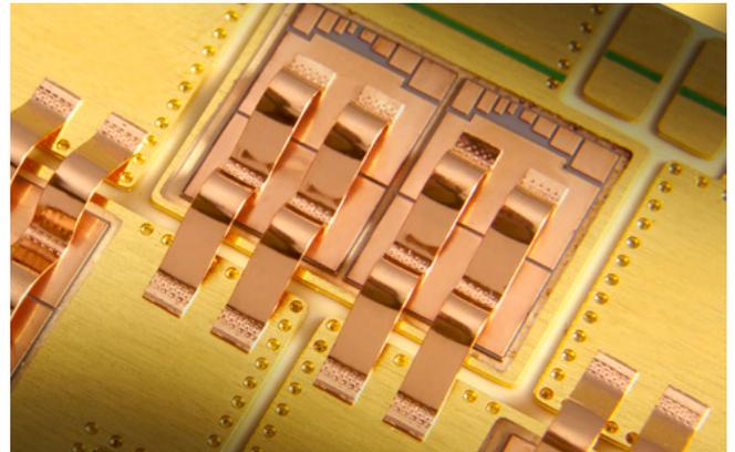
The conversion of chip contacting by aluminum wires, with copper wires or ribbons will significantly improve the potential and the reliability of power modules in the near future. Scientists at Fraunhofer ISIT have developed a copper deposition process on wafer level, and an automatic bonding process for copper ribbons.
