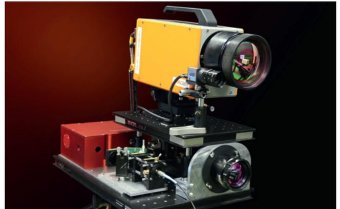
The Fraunhofer IAF application laboratory for IR spectroscopy detects and quantifies chemical reactions and substances with fast tunable quantum cascade lasers – in real time. As a result, various measurement tasks and application fields in the  $4 - 11 \mu\text{m}$  wavelength range can be covered:
