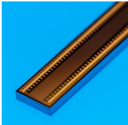
Fraunhofer IPMS develops micromachined ultrasonic components for various areas of application. These elements are uniquely capable of being integrated into CMOS processes as post-CMOS modules, paving the way for highly-miniaturized components with integrated evaluation electronics. Therefore, Fraunhofer IPMS is focused on the development of capacitive micromachined ultrasonic transducers (CMUTs).
