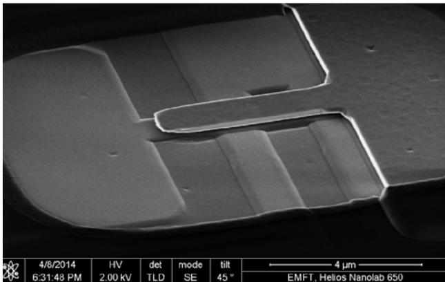
In the NanoFET project Fraunhofer EMFT is developing a miniaturized Nanogap Field Effect Transistor for highly sensitive sensors, together with industry partners. Due to the deployed nanostructures, even the slightest mechanical deflection causes a significant change in the electrical characteristics of the field effect transistor.
