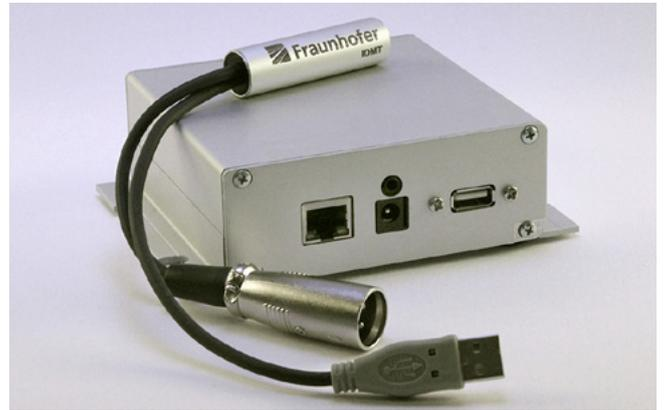
The Project Group Hearing, Speech and Audio Technology of Fraunhofer IDMT develops signal processing and hardware for computer-based acoustic monitoring in areas such as Industry 4.0, Security and Smart Cities/Smart Buildings. The hardware units for acoustic signal acquisition and processing can easily be integrated in existing cable-based or wireless sensor networks.
