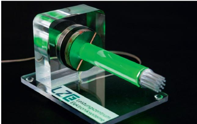
The reliable transfer of power in moving systems or harsh environments is required for a wide range of applications, such as in wind energy, Industry 4.0, healthcare, agriculture, or chemical industry. The inductive system, which was realized by the partners of the Leistungszentrum Elektroniksysteme (LZE) at the example of a ball bearing, offers bidirectional power and data transfer and improved safety as a wear-free alternative to failure-prone cable-based solutions.
