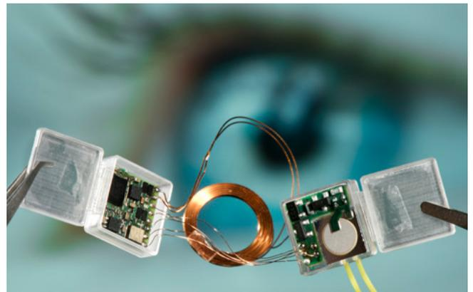
Elevated or too low intraocular pressure can cause problems with the eyesight and in the worst case even lead to blindness. There are no reliable long-term therapies to these ailments available today. In the “MIKROAUG” project funded by the BMBF, Fraunhofer EMFT, together with its industry partners, is developing a microfluidic system for treating such diseases of the eye. The microsystem, designed to be mounted directly on the ocular bulb, shall permanently stabilize the intraocular pressure.
