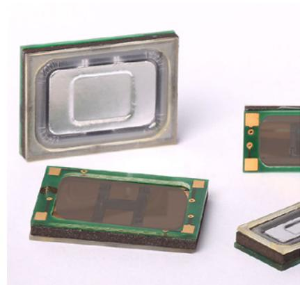
In collaboration with partners from industry and science Fraunhofer ISIT is developing a new generation of miniaturized loudspeakers, which are fabricated using silicon technology. In contrast to conventional electrodynamic micro speakers the new chip speakers are based on powerful piezoelectric MEMS drives and feature high energy efficiency and extremely low fabrication tolerances. Fields of application are mobile communication devices like tablets, smartphones and headphones.
