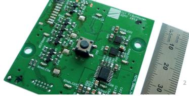
1, 2 At the Fraunhofer IDMT, arrays are developed with any number of microphones for a wide range of different applications. Fotos Fraunhofer IDMT
