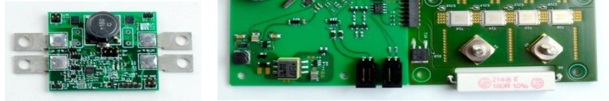
Picture 1: Cell management controller (CMC) and module / battery management controller (MMC / BMC)
