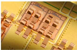
The conversion of chip contacting by aluminum wires, with copper wires or ribbons will significantly improve the potential and the reliability of power modules in the near future. Scientists at Fraunhofer ISIT have developed a copper deposition process on wafer level, and an automatic bonding process for copper ribbons.
