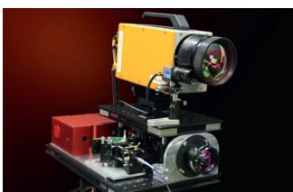
The Fraunhofer IAF application laboratory for IR spectroscopy detects and quantifies chemical reactions and substances with fast tunable quantum cascade lasers – in real time. As a result, various measurement tasks and appplication fields in the
