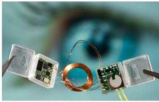
Elevated or too low intraocular pressure can cause problems with the eyesight and in the worst case even lead to blindness. There are no reliable long-term therapies to these ailments available today. In the "MIKROAUG" project funded by the BMBF, Fraunhofer EMFT, together with its industry partners, is developing a microfluidic system for treating such diseases of the eye. The microsystem, designed to be mounted directly on the ocular bulb, shall permanently stabilize the intraocular pressure.
