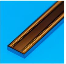
Fraunhofer IPMS develops micromachined ultrasonic components for various areas of application. These elements are uniquely capable of being integrated into CMOS processes as post-CMOS modules, paving the way for highlyminiaturized components with integrated evaluation electronics. Therefore, Fraunhofer IPMS is focused on the development of capacitive micromachined ultrasonic transducers (CMUTs).
