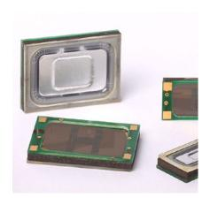
In collaboration with partners from industry and science Fraunhofer ISIT is developing a new generation of miniaturized loudspeakers, which are fabricated using silicon technology. In contrast to conventional electrodynamic micro speakers the new chip speakers are based on powerful piezoelectric MEMS drives and feature high energy efficiency and extremely low fabrication tolerances. Fields of application are mobile communication devices like tablets, smartphones and headphones.
