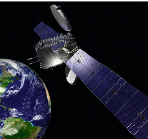
Geostationary satellites orbit the Earth once a day along the equator. © SES – www.ses.com
