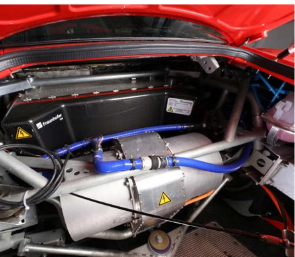
A look under the hood gives us a clear view of the battery system and the double drive unit developed by Fraunhofer IISB. © Fraunhofer IISB / Kurt Fuchs
