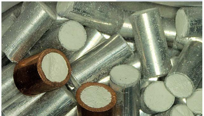
The chemical industry uses large quantities of packing materials. To protect the millimeter-scale particles against abrasion, Fraunhofer IKTS encapsulates them in a layer of metal that boosts their thermal conductivity by a factor of five. © Fraunhofer IKTS
