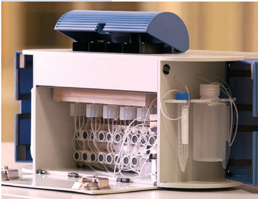
The finished "laboratory": assay processor for fully automated processing of several BioChip cartridges. © Fraunhofer IZM
