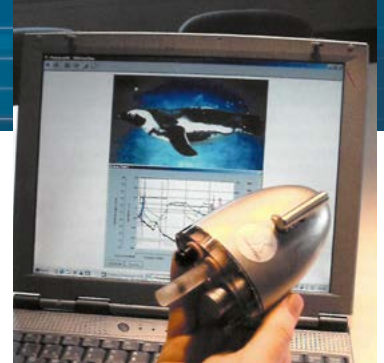
The miniaturized tachograph for marine life such as seals and penguins contained a variety of sensors for simultaneous measurement of data such as pressure, temperature, pH value and brightness. © Fraunhofer IZM
