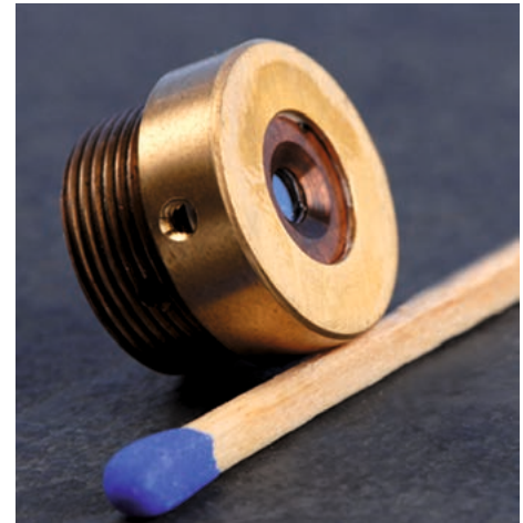
The basis of the new laser technology: a semiconductor chip for the wavelength range between two and three micrometers, fitted in a special heat sink. © Fraunhofer IAF
