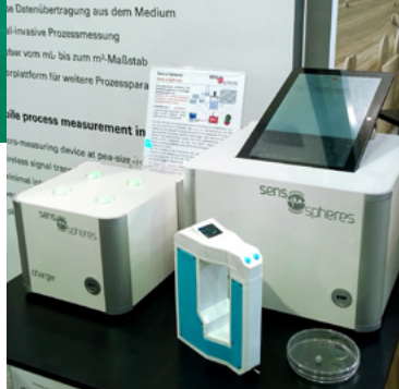
Sens-o-Spheres demonstrator. The picture shows the charging station, the base station, the Sens-o-Spheres and a handheld to apply the spheres sterile.
