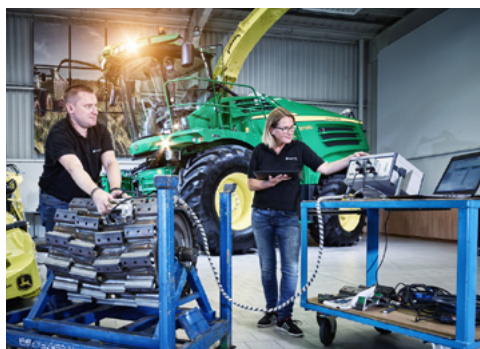
Weld seam testing on the blade holder of a John Deere forage harvester using LinScanDuo 2.0. © Fraunhofer IZFP / Uwe Bellhäuser
