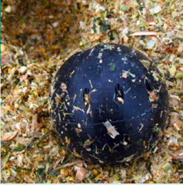
A ball with hidden features. A very robust housing protects the sensors against the high pressure in the compressed silage. © Fraunhofer IZM
