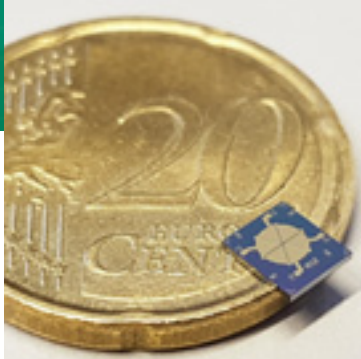
Size comparison: The chip of a MEMS loudspeaker on a 20-cent coin. © Fraunhofer ISIT
