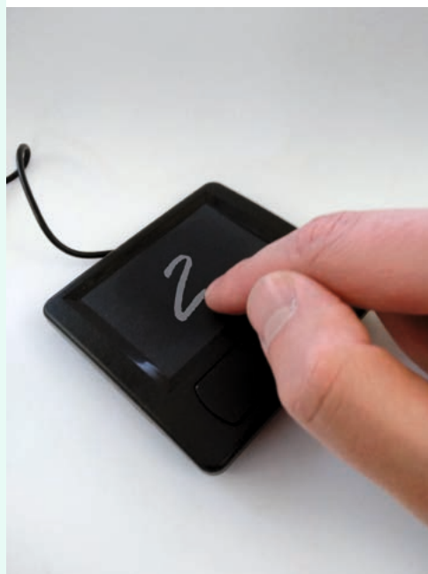
AlfES demonstrator for handwriting recognition: the numbers are drawn by hand on this touchpad and then recognized and output by AlfES on the microcontroller.
