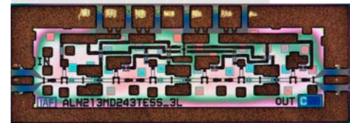
Amplifier circuit with MOSHEMT transistors at 243 GHz. © Fraunhofer IAF
