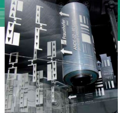
Roll-to-roll printing of antennas. © Fraunhofer ENAS
