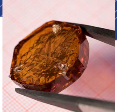
Aluminum nitride crystal as semiconductor base material for power electronic devices.
