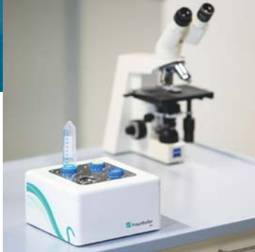
The TissueGrinder enables gentle tissue dissociation. © Fraunhofer IPA
