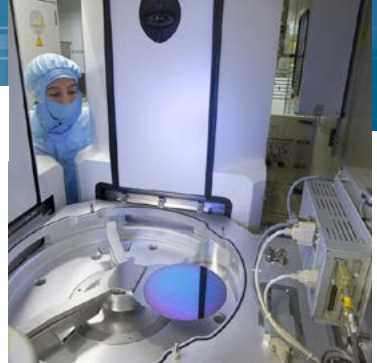
Thermally assisted chemical vapor deposition on an 8" wafer.
